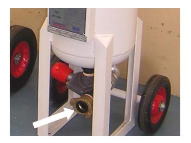
Connect the blasting hose to the outlet coupling on the Micro-valve
