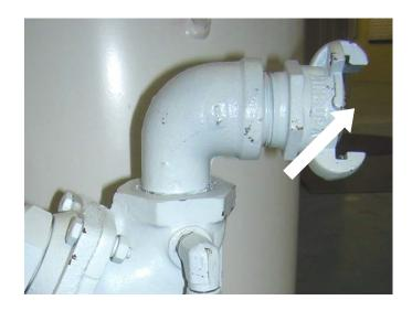
Connect the supply air hose to the inlet connection. Some versions may have an inlet moisture filter
